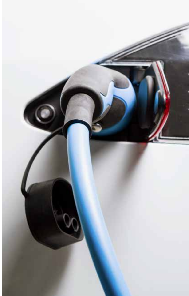
Electric vehicles must have a standard plug-in connector to charge from standard power points.
