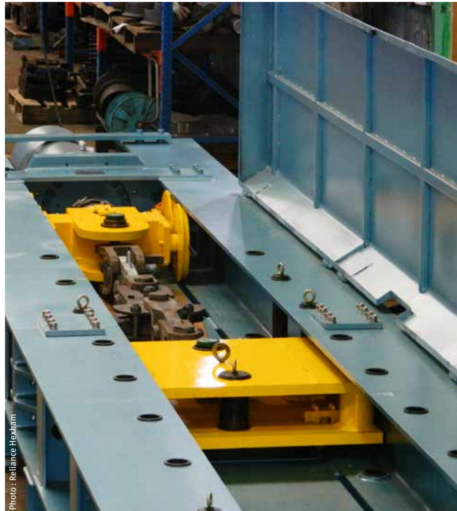
The 200T Test Rig, which is used to conduct proof load and destructive tests for design validation.
